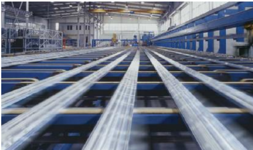
The 1,900 tonne extrusion line operated by EUROMETAL SA.
